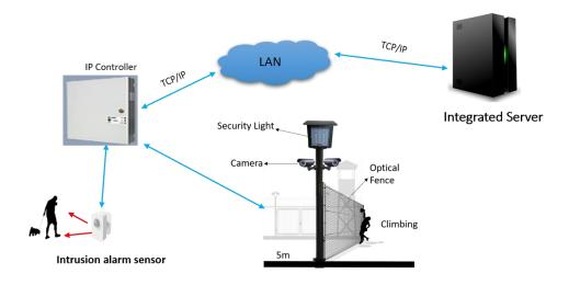
Intrusion alarm system having PIR sensors in equipment room and one more in any critical area where user wants to monitor any movement in any critical areas. Alarm will be raised based on Integrated with centralised alarm management system.
