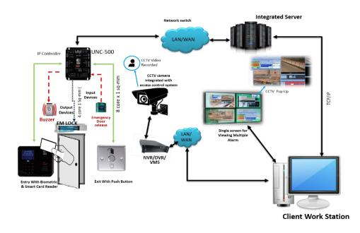
There will be a CCTV integrated to alarm points of any system enabling POP up of camera system in central software in case of alarm. There should be a provision to connect more than one camera to a single alarm point as many times alarm point cannot be covered by a single camera view.
